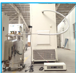
LN 2 /CO 2 backup system
